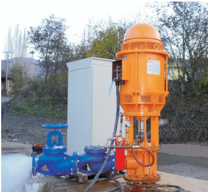
Vertical turbine pumps are used to pump geothermal water from underground to surface. At beginning, these pumps were designed for narrow and deep wells. Later, they were improved for different applications; one of them is geothermal application.
