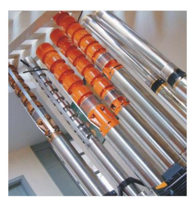
A submersible pump is turbine pump close-coupled to a submersible electric motor. Both pump and motor are suspended in the water, thereby eliminating the long drive shafts and bearing retainers required for a deep well turbine pump. Because the pump is located above the motor, water enters the pump through a screen located between the pump and motor. The pump curve for a submersible pump is very similar to a vertical turbine pump.
