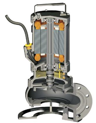
Sewage pumps are used to pump solids and semi-solids in a variety of commercial, industrial, maritime, municipal and wastewater treatment applications.
