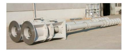
Vertical turbine pumps are firstly invented by Mr. M. Layne and adapted for use in cased wells or where the water surface is below the practical limits, where other pumps cannot do the same job. Vertical turbine pump efficiencies are comparable to or greater than most centrifugal pumps.
